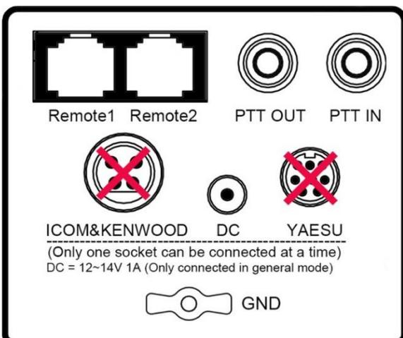
If you use transmitters other than Yaesu, ICOM or Kenwood with an external DC power supply connected, when you press the "POWER" button on the front panel to start, this mode will be set automatically. The voltage of external power supply shall be in the range of 10-15v, and the maximum working current shall not be less than 1A. Other cable connections are described below.
