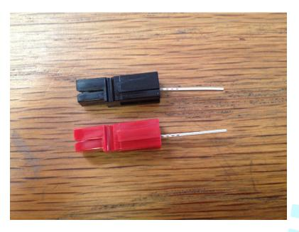
6. Pair up, the shells as shown, one black and one red. The shells will pair up in many ways so make sure that you get them right – as shown in the photograph. This is the "standard way" of using PowerPole connectors for ham radio use.
